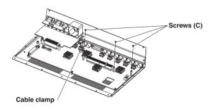
⑥ Insert the HD analog board from the inside of the rear panel, and insert it along the guide rail for the connector. (Insert it securely and completely.)
